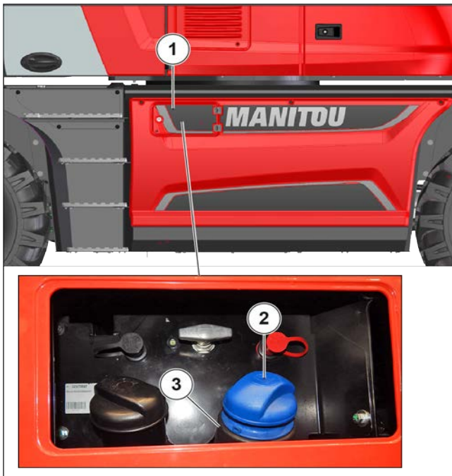
Figure 149: Checking DEF liquid level
