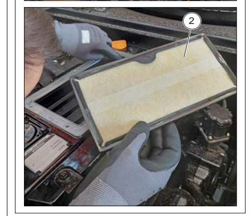
Figure 209: Replacement of the crankcase filter of the engine breather
