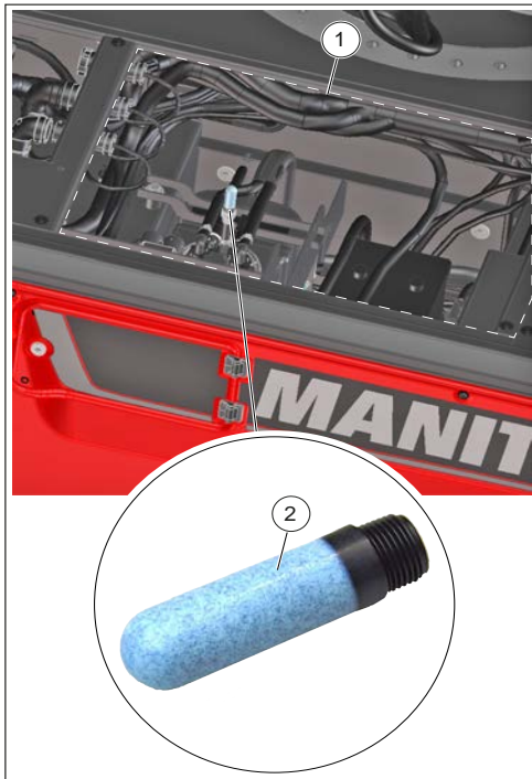
Figure 205: Replace the "DEF" tank breather
