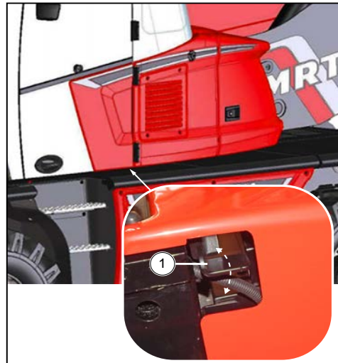
Figure 61: Door window release lever from outside cabin
