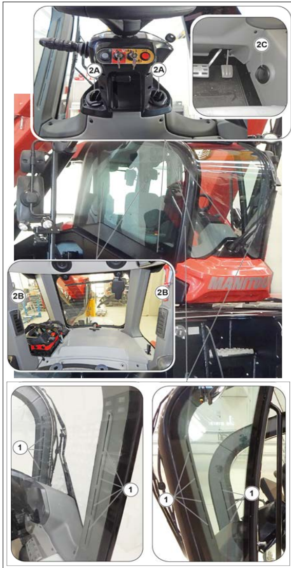
Figure 62: Demisting diffusers and heating air vents
