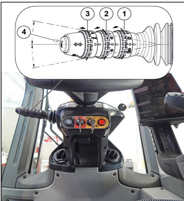
Figure 54: Control lever for lights, horn, indicator lights and wipers
